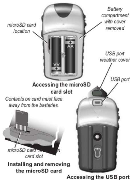
*Installing the batteries and a microSD card*
