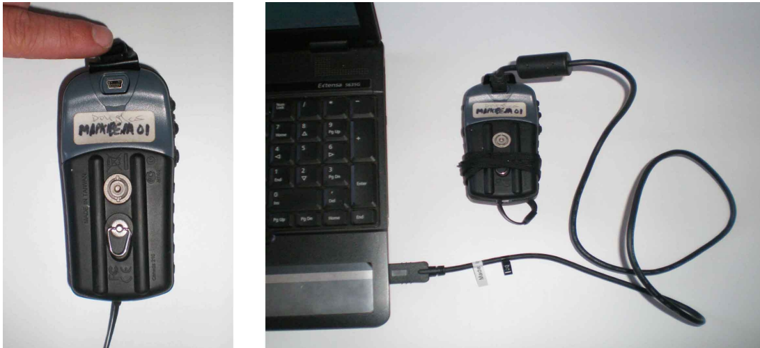
Connecting the GPS unit to the computer
